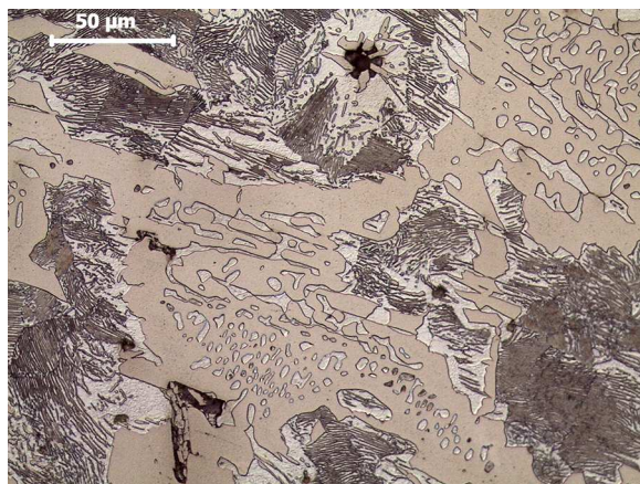
Figure 6. Rhizon steel ingot: microsection at X in Fig. 4, at higher magnification, showing pearlite and ledeburite with slag inclusions. Reproduced by kind permission of M. Biborski and J. Stępiński. Map: iron working sites during the Roman period (after Pleiner, 2000, fig.12).
